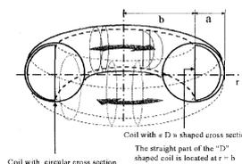
Figure 6: Double D-shaped toroid [29]
