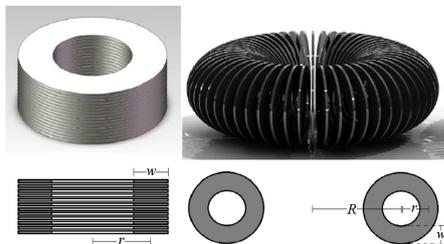
Figure 5: Solenoid and Toroid configurations [28]
